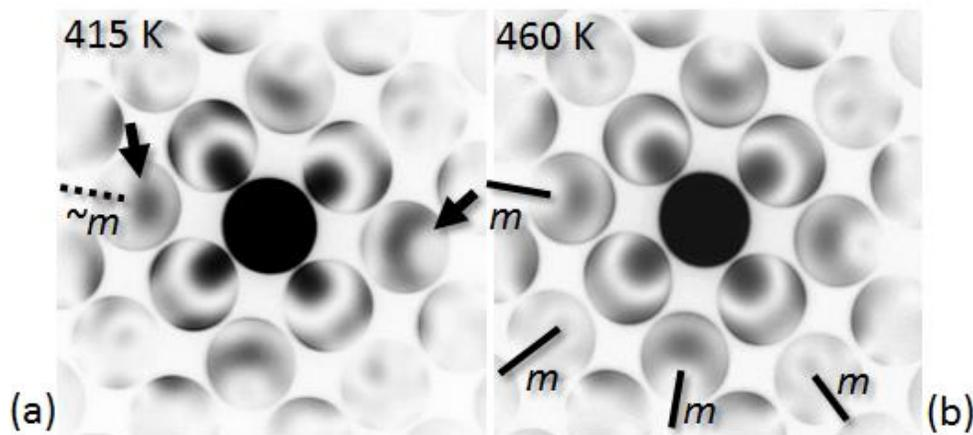
**Figure 1.** Energy-filtered [100] CBED patterns of the cubic phase of BaTiO<sub>3</sub> taken at specimen temperatures of (a) 415 K and (b) 460 K. The pattern (a) exhibit clear breaking of the fourfold rotation symmetry expected from the cubic phase, while the pattern (b) shows almost the fourfold rotation symmetry.
