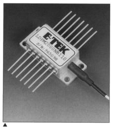
Laser Diode Power Module: The 1550 nm LDPM from E-TEK Dynamics delivers more than 20 mW of power and is designed for high-power continuous-wave optical sources for analog applications using an external modulator. The device includes a distributed feedback laser diode, thermoelectric cooler, monitor photodiode, isolator, and pigtailed single-mode or polarization-maintaining fiber in a hermetically sealed 14-pin dual-in-line or butterfly style package.
