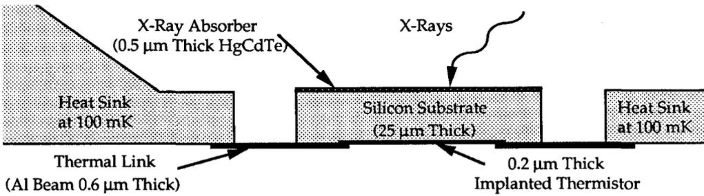
Figure 1. A side view of an X-ray calorimeter (not to scale). When an X-ray hits the absorber (HgCdTe), the photon energy is converted to thermal energy. The resulting temperature rise can be measured by the ion-implanted thermistor. Aluminum beams provide thermal and electrical links.
