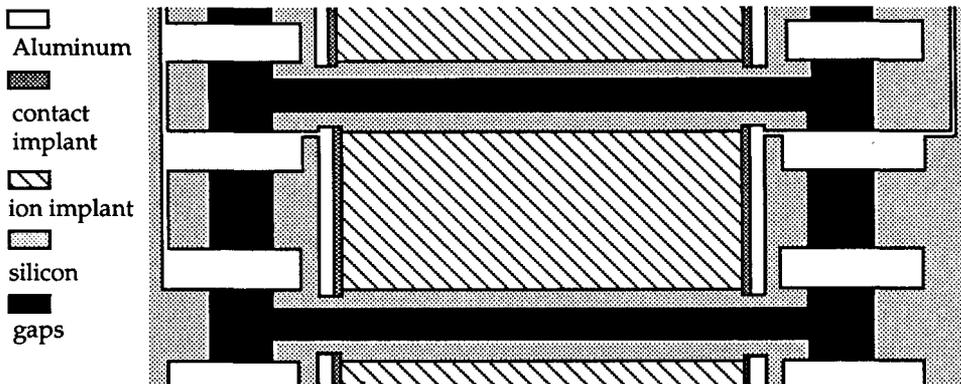
Figure 2. A single detector element of a testing array
