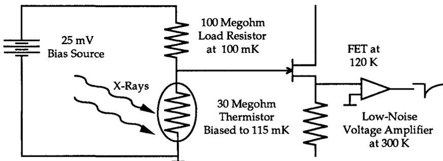
Figure 3. An electrical circuit used to run a calorimeter.
