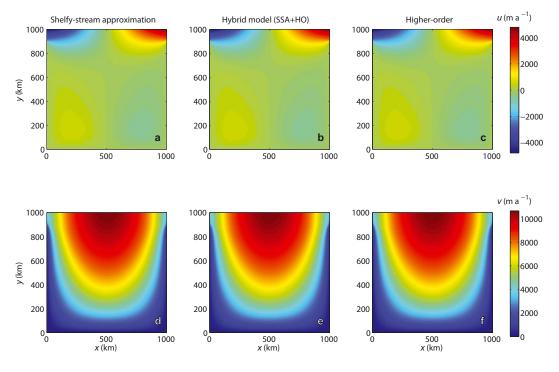
**Fig. 5.** Top view of velocity components of a square ice shelf for three ice flow models: SSA, HO and a hybrid SSA/HO model. (a) u for SSA; (b) u for hybrid; (c) u for HO; (d) v for SSA; (e) v for hybrid; (f) v for HO.
