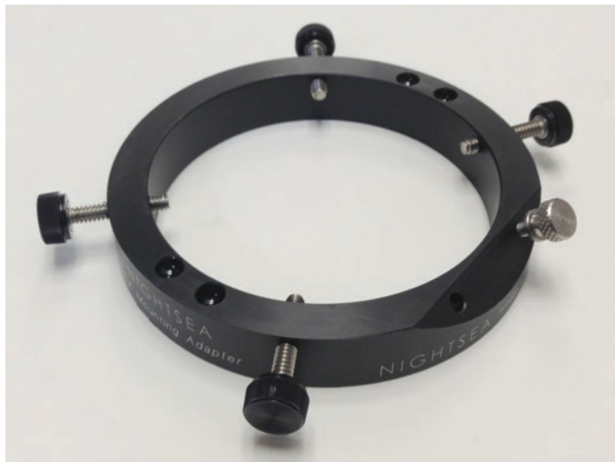
Figure 3: The SFA adapter ring has an inside diameter of 67 mm, enabling it to fit most stereo microscopes without a special adapter. The thumbscrews can adjust to fit microscopes with diameters down to 50 mm. The adapter ring holds four small neodymium magnets for attachment of the barrier filters.
