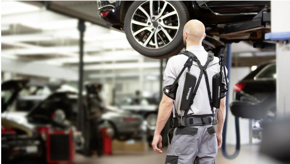
Figure 1. Passive exoskeleton Ottobock Paexo
