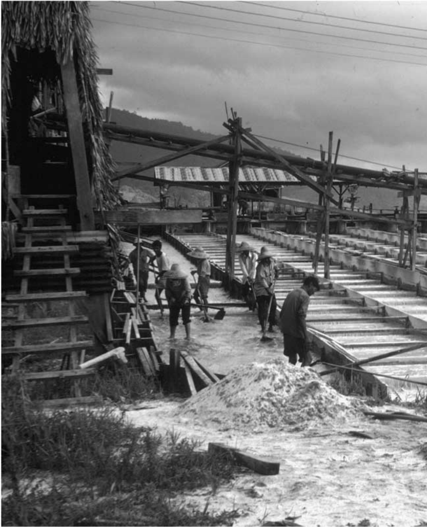
Figure 4. Chinese miners working on a palong at a Chinese gravel pump tin mine in the Kinta Valley (Malaysia), 1978.
