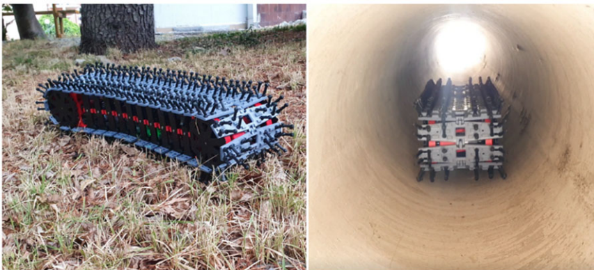
Figure 15. Experimental tests: locomotion on grassy and leafy soft terrain (left) and inspection of a pipe with diameter of 300 mm (right).
