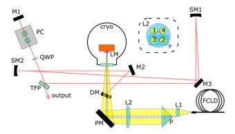
**Figure 2.** Schematic of the laser setup. The dashed box inset shows the hit points of the pump beam on L2 and P. Cryo, high-vacuum cryostat; DM, dichroic mirror; FCLD, fiber-coupled laser diode; L1 and L2, lenses; LM, active mirror laser medium; M1, M2, M3, turning mirrors; P, retro-reflector prism; PC, Pockels cell; PM, pump turning mirror; QWP, quarter wave plate; SM1 and SM2, spherical mirrors; TFP, thin-film polarizer.
