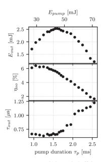
**Figure 3.** Output energy  $E_{\rm out}$ , optical-to-optical efficiency  $\eta_{\rm oo}$  and full width at half maximum output pulse duration  $\tau_{\rm out}$  as functions of the pump pulse duration in Q-switch operation. The pump diode was operated at 28 W peak power and 1 Hz repetition rate. The secondary x-axis on top indicates the total pump energy  $E_{\rm pump}$  applied.
