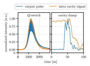
**Figure 4.** Temporal pulse shapes of the intracavity signal and the output pulse at maximum energy.
