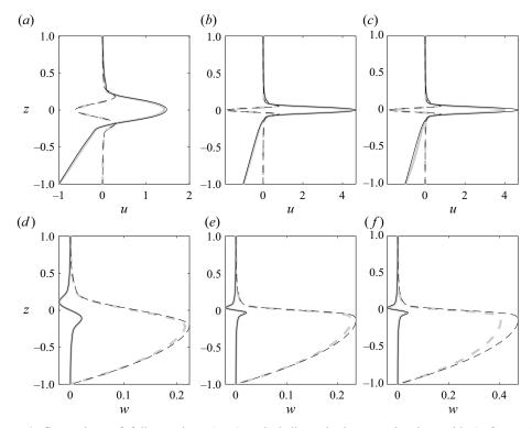
Figure 4. Comparison of full equations (grey) and shallow elastic approximation, with (a,d)  $\alpha=0.5$ ,  $\varepsilon=10^{-3}$ , (b,e)  $\alpha=0.5$ ,  $\varepsilon=10^{-5}$  and (c,f)  $\alpha=1$ ,  $\varepsilon=10^{-5}$ . For all cases we have set  $\beta=0.2$  and R=1. Note the good agreement even at moderate  $\alpha=1$ . Solid and dashed lines indicate the real and imaginary components of the solution, respectively.
