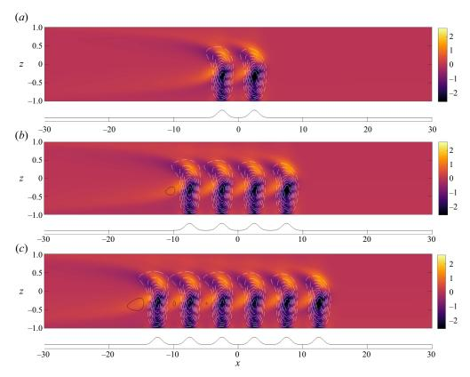
Figure 6. Response to a series of  $n \in \{2, 4, 6\}$  Gaussian bumps with  $l_x = 1$  in a viscoelastic flow with W = 200, R = 1 and  $\beta = 0.5$ . The bumps are spaced apart by  $5l_x$  in the streamwise direction. Colours show the spanwise vorticity perturbation, lines are the perturbation streamfunction (solid black positive, dashed white negative).
