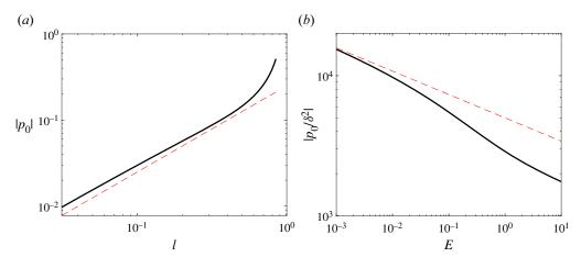
Figure 9. Pressure and vorticity amplification as a function of elasticity, obtained from calculations at  $\varepsilon = 10^{-6}$ ,  $\beta = 0.5$ . The red lines indicate (a)  $p \sim l(E) = \sqrt{E}$  and (b)  $\omega \sim E^{-1/6}$ .
