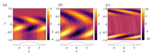
Figure 3. Vortical response to monochromatic surface roughness  $h(x) = \cos \alpha x$ , with  $\alpha = 0.5$ : (a) W = 200,  $\beta = 0.2$ , R = 1; (b)  $\beta = 0.5$ , R = 100, W = 100; (c) W = 200, W = 200. Colours are spanwise vorticity perturbations, lines the perturbation streamfunction.
