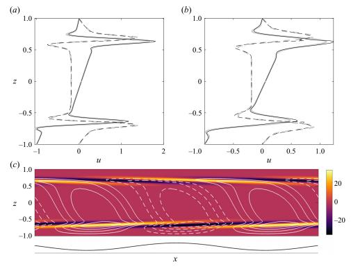
Figure 8. Composite (black) and numerical (grey) solution in the shallow elasto-inertial regime: (a) E = 0.2,  $\varepsilon = 10^{-3}$ ,  $\beta = 0.5$ ; (b) E = 0.5,  $\varepsilon = 10^{-3}$ ,  $\beta = 0.8$ . Solid and dashed lines indicate the real and imaginary components of the solution, respectively. (c) The vorticity field (colours) and streamfunction (lines) corresponding to the E = 0.2 case.
