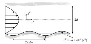
Figure 1. Schematic of the flow configuration considered in this paper, with variables shown in their dimensional form. The problem is non-dimensionalised by the channel half-height, d, and the wall shear rate,  $\dot{\gamma}$ , of the base-flow velocity. A monochromatic surface topography is shown for illustration.
