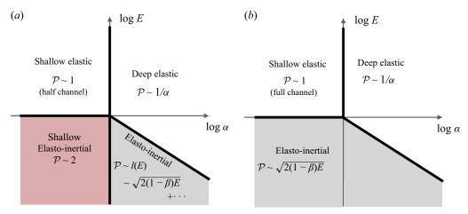
Figure 10. Phase diagrams for (a) the wavy channel and (b) wavy Couette flow from Page & Zaki (2016). Also included is an estimate of the penetration depth,  $\mathcal{P}$ , of the vorticity perturbation induced at the lower wall. Note that the diagonal line in the bottom right quadrant indicates  $1/\alpha \sim \sqrt{2(1-\beta)E}$ .
