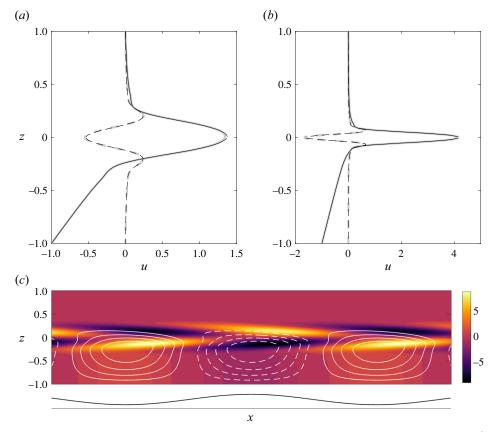
Figure 5. Composite (black) and numerical (grey) solution in the shallow elastic regime: (a)  $\varepsilon = 10^{-4}$ ; (b)  $\varepsilon = 10^{-6}$ . In both cases R = 1 and  $\beta = 0.8$ . Solid and dashed lines indicate the real and imaginary components of the solution respectively. (c) The vorticity field (colours) and streamfunction (lines) corresponding to the  $\varepsilon = 10^{-4}$  case.
