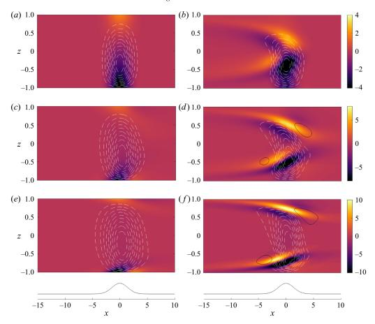
Figure 2. Response to Gaussian bump with  $l_x = 2$  in (a,c,e) Newtonian and (b,d,f) viscoelastic flows with W = 200 and  $\beta = 0.5$ . The Reynolds number is matched between the Newtonian and viscoelastic calculations and increases from top to bottom,  $R = \{1, 200, 1000\}$ . Colours show the spanwise vorticity perturbation, lines are the perturbation streamfunction (solid black positive, dashed white negative).
