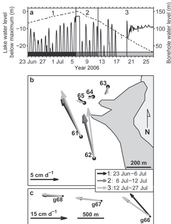
**Fig. 2.** (a) Measured lake water level (dashed) and water level in borehole bh6 (solid) during the drainage of Gornersee in 2006. The drainage event is subdivided into the three intervals 1–3, as indicated by the shaded bars and vertical lines (thin solid). (b) Vector plot of horizontal flow velocities observed in the ice dam during the three intervals 1–3. (c) Vector plot of horizontal flow speeds observed down-glacier of the ice dam during the three intervals 1–3.
