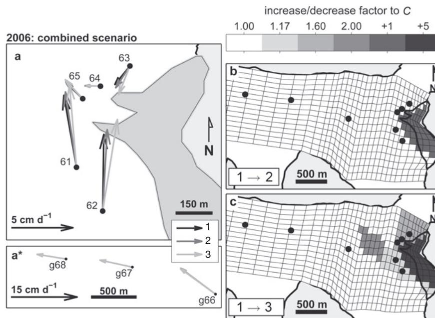
**Fig. 7.** (a) Computed flow velocities for a combined scenario in 2006. The velocity of interval 1 includes the full lake water pressure, which is removed in two steps, of  $-6$  and  $-18$  m in intervals 2 and 3, respectively. (b, c) Relative changes applied to the initial  $C$ -configuration (Fig. 4b) to reproduce the velocities of intervals 2 and 3. The greyscale referenced to '+1' and '+5' indicates that  $C$  was set from zero ( $\sim 10^{-8}$ ) to 1 or 5.
