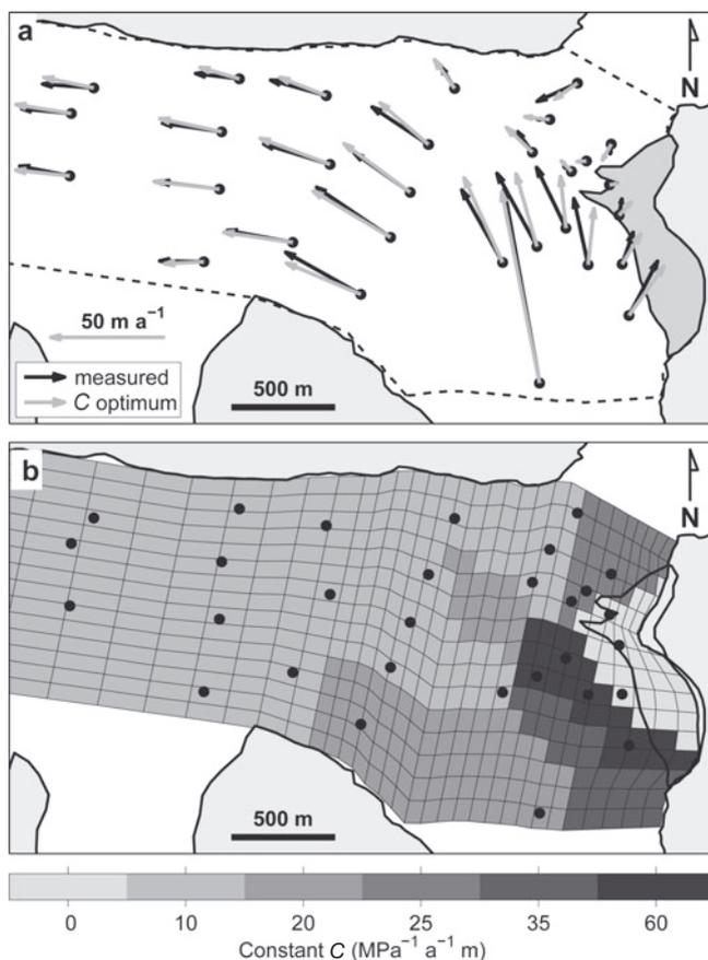
**Fig. 4.** (a) Comparison of measured (black) and optimum calculated (grey) summer horizontal flow velocities at a set of  $N = 30$  stakes. The model domain outline is indicated by a dashed curve. (b) View from above of the bed-layer elements and the spatial settings of the constant  $C$  used for the flow-field computation shown in (a). The black dots correspond to the velocity measurement markers as in (a), and the outline of Gornersee is indicated.
