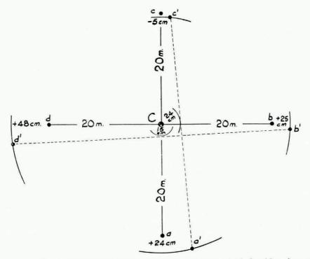
Fig. 2. An attempted reconstruction of Pfaff's differential flow measurements. Original position of posts indicated by a, b, c and d. Final position a', b', c' and d'.
