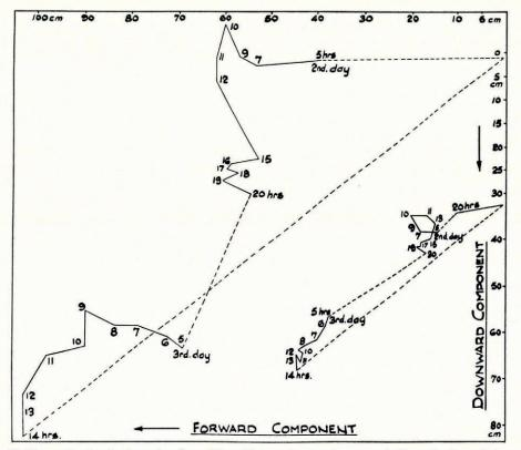
Fig. 1. Pfaff's graphs showing irregular flow of firn. The numbers on the curves indicate the time of day on each of 3 days
