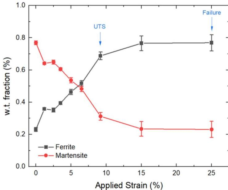
**Figure 1.** Strain-induced phase transformation of a 4130 pressure vessel steel determined from analyzing neutron diffraction patterns. Weight fractions of ferrite (black) and martensite (red) are shown as a function of applied strain. The ultimate tensile strength (UTS) sample and failure sample are indicated by blue arrows.
