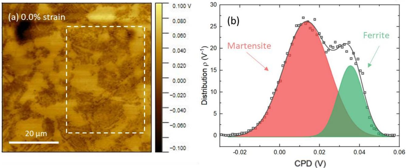
**Figure 2.** (a) Scanning Kelvin probe force microscopy (SKPFM) image of an un-strained 4130 steel sample. (b) Histogram of the potential landscape measured from the area indicated by the white-dashed line box in the SKPFM image. Analysis of the bimodal histogram reveals a ferrite / martensite ratio similar to what was observed from neutron diffraction (77% / 23%).
