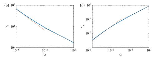
Figure 4. Plots of  $r^*$  and  $z^*$  as functions of  $\alpha$  for Bo = 0.1. The thick blue lines are the exact solutions, obtained using the numerical scheme of § 3. The thin red lines provide the pancake approximations (5.5*b*) and (5.6), valid for  $\alpha \ll Bo^{3/2}$ . The dashed red lines are the spherical-cap approximations (6.23*a*) and (6.24), valid for  $Bo^{3/2} \ll \alpha \ll 1$ .
