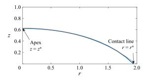
Figure 1. Drop shape for  $\alpha = 45^{\circ}$  and Bo = 1, depicted using the dimensionless (*r*, *z*) interface coordinates (shown on an equal scale). The thick blue line is produced by the numerical scheme of § 3. The thin red line is the asymptotic approximation in the distinguished limit (6.1).
