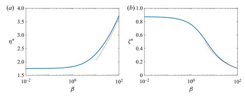
Figure 3. Plots of  $\eta^*$  and  $\zeta^*$  as functions of  $\beta$ . Thick blue lines: solution of (6.13) and (6.17). Thin red lines: pancake limits (6.19). As  $\beta \to 0$  the numerical results agree with the approach to the spherical-cap limits  $\eta^* = (16/3)^{1/3} \approx 1.7472$  and  $\zeta^* = (2/3)^{1/3} \approx 0.8736$ ; see (6.23) and (6.24).
