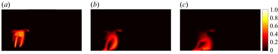
Figure 2. Temporal evolution of the solute plume for R = 3 , Ra = 9000 , a/b = 3 and f_L = 0.001 . The plume is shown at dimensionless times (a) t = 0.3 , (b) t = 0.6 and (c) t = 0.9 . These three snapshots in time show the complex nonlinear interplay between viscous and density fingering mechanisms that can lead to folding (e.g. vortex-like structure) of the plume. This observed folding dynamics is unique to the specific model configuration investigated in this work.
