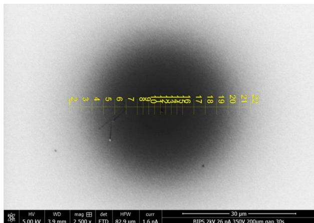
**Figure 3:** SE image after Ar ion milling at 350V, 200 um gap, 30s, electron beam scan mode. The points indicate the EDX measurement positions. In the center point 16 nm Pt has been sputtered (from initial 23 nm).
