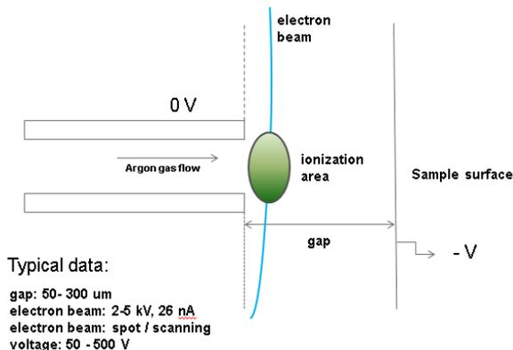
**Figure 1:** Schematic set up of an in-situ low energy ion source. The field  $-V/\text{gap}$  induces acceleration of ions towards the sample surface.
