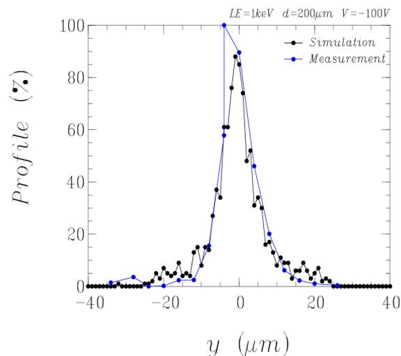
**Figure 4:** Example of simulated ion beam profile (black) and measured profile (blue) for a 100 V ion energy and 200 um gap. Electron beam in spot mode.
