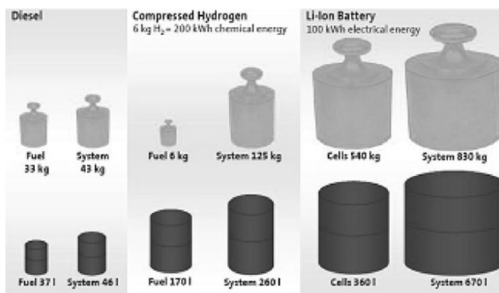
Figure 3. Comparison of mass and volume for energy storage with hydrogen, batteries, and fuel (Von Helmholt and Eberle, 2007).
