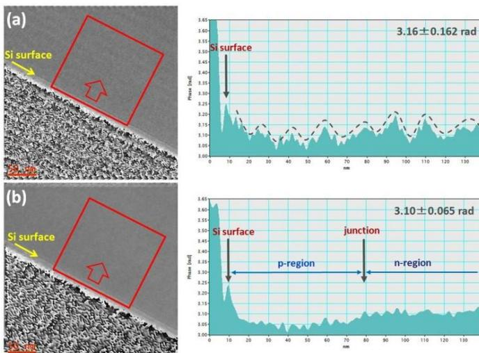
**Figure 3.** Electron holography for a 1D Si/Si p-n junction with very low doping level. (a) the phase image reconstructed from a common hologram with Fresnel fringes, the profile from it showing the influence of the Fresnel fringes on the phase; (b) the phase image from a hologram using only center part of the interference band, no Fresnel fringe effect so its profile revealing p-n junction location.
