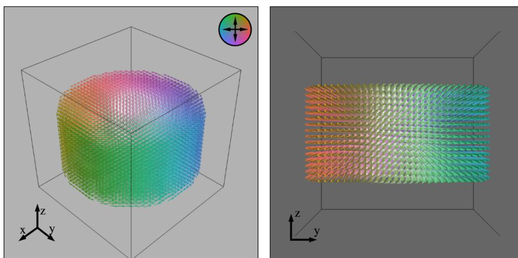
**Figure 1.** Reconstructed magnetization distribution of a magnetic vortex state calculated from two tilt series of simulated magnetic phase images generated for maximum tilt angles about the x and y axes of  $\pm 90^\circ$  and an angular sampling of  $5^\circ$ . The color wheel encodes the magnetization direction in the xy plane, while white arrows point in the positive z direction.
