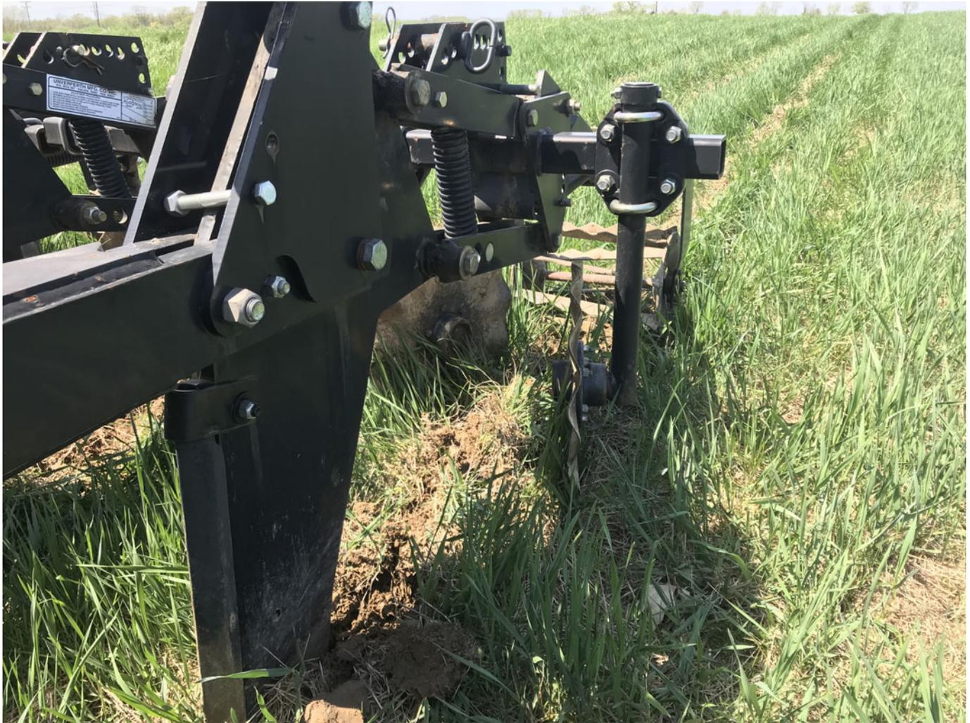
**Fig. 2.** Strip-tillage treatment being applied using Unverferth Zone Builder Subsoiler Model 122.
