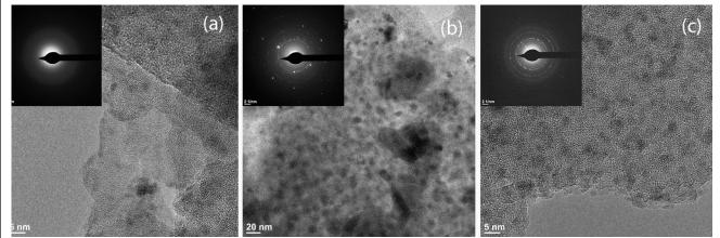
**Figure 1.** TEM images and corresponding diffraction patterns for different composites: 5%Ni-SiO<sub>2</sub> (a), 30%Ni-SiO<sub>2</sub> (b) and 5%NiO-SiO<sub>2</sub> (c)
