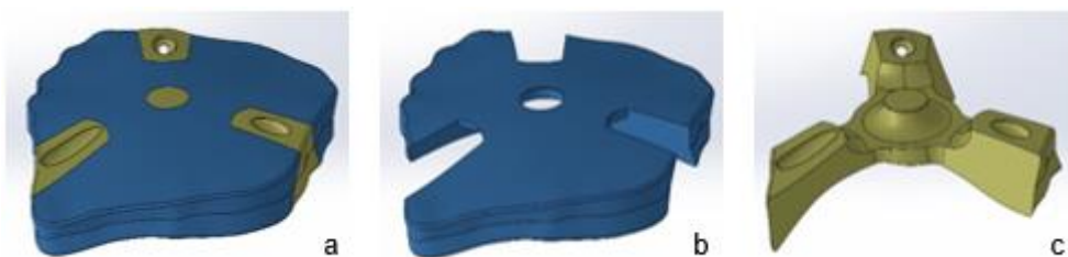
Figure 5: (a) Designed hybrid structure of the implant: completely; (b) Filling structure; (c) Bearing structure
