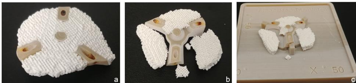
Figure 7: Additively manufactured hybrid implant: (a) Specimen 1 - not destroyed; (b) Specimen 2 - destroyed; (c) Specimen 2 on the building plate with negative - destroyed
