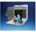
The MicroFlow II is a Class 1 ductless carbon-filtered workstation equipped with activated carbon filtration. It is completely self-contained with integral recessed work surface to contain spills. A clear hood surrounds the work area and includes a hinged viewing sash for user protection. The sash can be conformed for use with a microscope. Variable speed fan control allows for
