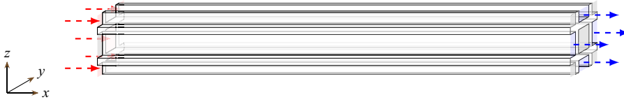
Figure 1. The four-channel set-up of one central inflow (red) channel with fractions of surrounding inflow (red) and outflow (blue) channels separated by porous walls. Grey, no-slip walls. The sketch is scaled for improved visual clarity.
