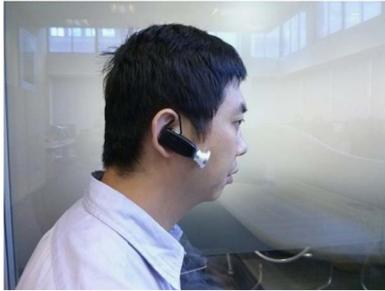
**Fig. 1.** Micro-camera device used in this pilot study, as worn over the ear.
