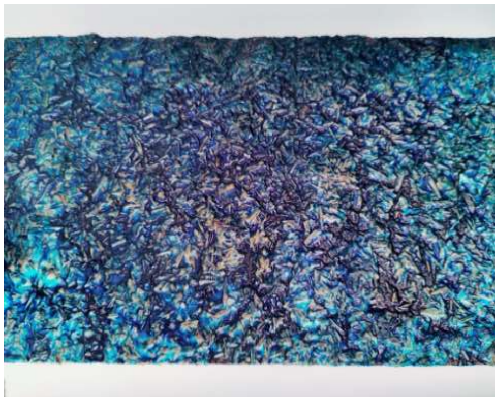
Figure 9: Mycelium leather samples measuring 30 cm x 48 cm grown using Ecovative living material, treated with blue algae solution using a spray-on application.
