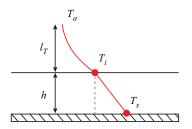
Figure 5. Sketch of the one-dimensional heat transfer model used to estimate the time needed for the interface temperature  $T_i$  to reach the liquid boiling temperature  $T_b$ .
