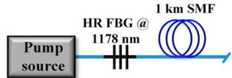
Figure 10. The experimental setup of 1178 nm Random laser.
