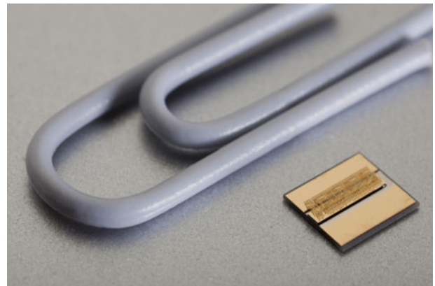
Figure 3. 400\ \mu\text{m} high-power QCW laser for kW-pump modules. The chip is mounted on a plated AlN substrate. The size of the submount is 4\ \text{mm} \times 4.5\ \text{mm} \times 0.4\ \text{mm} .
