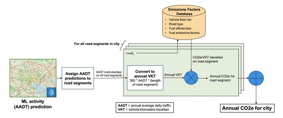
Figure 2. Emissions calculation overview, from ML-predicted AADT to emissions estimate for an entire city.
