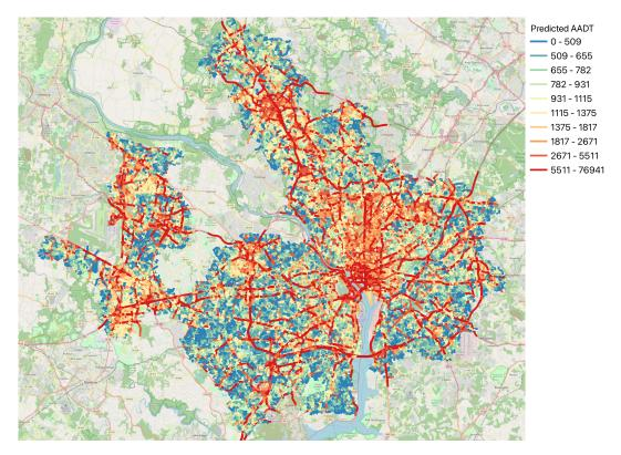
*Figure 3.* Example ensembled AADT predictions for the greater Washington, DC area. AADT units are vehicles per day. Map data from OpenStreetMap (*Haklay and Weber, 2008*).
