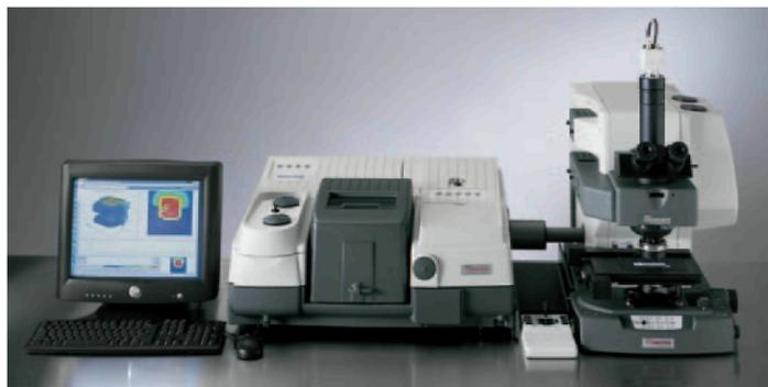
Figure 1. Nicolet Continuum XL Imaging Microscope with Nicolet 6700 FT-IR Spectrometer and OMNIC Atlas software
