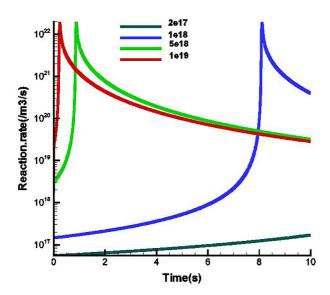
**Figure 5.** Temporal evolution of the reaction rate. The curves correspond to different initial values of the alpha particles produced by the  $\mu$ CF in the spark part of the device: (a) red  $10^{19}$  m<sup>-3</sup>, green  $5 \times 10^{18}$  m<sup>-3</sup>, blue  $10^{18}$  m<sup>-3</sup> and deep green  $2 \times 10^{17}$  m<sup>-3</sup>.
