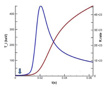
**Figure 4.** Temporal evolution of the reaction rate, and plasma ion temperature. The blue arrow indicates the end of operation of the  $\mu$ CF in the spark fusion part of the device which correspond to 1  $\mu$ s.
