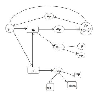
Figure 1. Full description of muon catalysis fusion cycle.
