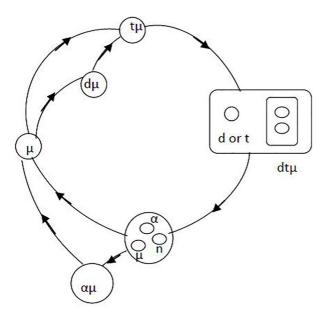
Figure 2. Reduced  $\mu$ CF catalyzed cycle.
