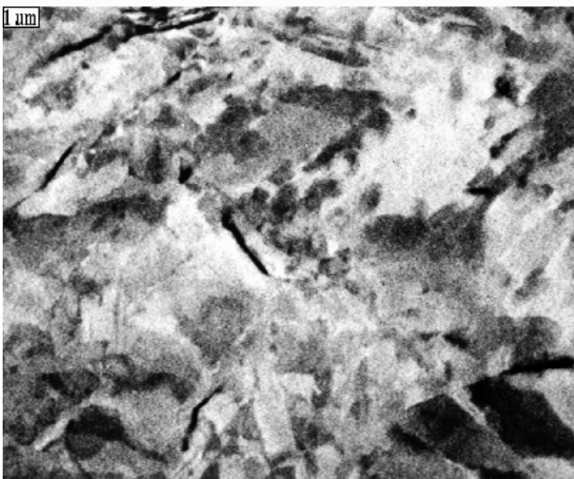
Fig. 5. IF Steel - Drawn Cup Sidewall.
