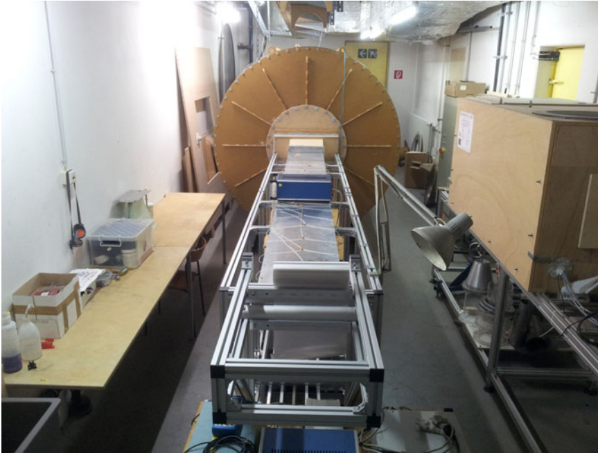
FIGURE 27. Experimental facility at the Lehrstuhl für Strömungsmechanik for study of viscous drag reduction by surface embedded grooves.
