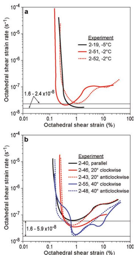
**Fig. 3.** Creep curves for samples experimentally deformed at  $-5^{\circ}\text{C}$  (a) and  $-2^{\circ}\text{C}$  (a, b) in combined compression and shear with a compressive stress of 0.22 MPa and shear stress of 0.4 MPa. (a) Polycrystalline ice in experiments 2-19, 2-51 and 2-52. (b) Columnar ice with layering parallel (2-40), inclined  $20^{\circ}$  and  $40^{\circ}$  clockwise (2-46, 2-55) and  $20^{\circ}$  and  $40^{\circ}$  anticlockwise (2-43, 2-48) to the  $x_1x_2$  plane.
