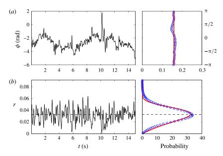
FIGURE 3. A time series and probability density of the centre of pressure: angular (*a*) and radial (*b*) position. Symbols in the probability density (right) correspond to experimental data and solid lines to theoretical model predictions. Dashed line: mean radial value indicating the broken  $\Re_{\pi}$  symmetry.
