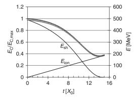
Fig. 18.4. The calculated dependencies of  $E_{\rm ion}$ ,  $E_{\rm sh}$  and  $E_{\rm C}$  (lower line with triangle symbols) on t. The upper line with diamond symbols shows the ratio of the energy deposition in the calorimeter to its maximum value (without leakage). Even when the charge exchange occurs in the very beginning of the calorimeter, some part of the energy leaks through the rear side.
