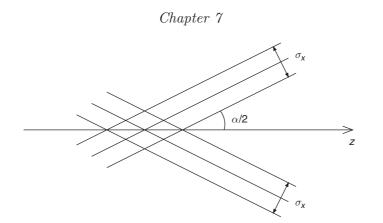
Fig. 18.2. Illustration of the vertex resolution  $\sigma_z$  as derived from the track resolution  $\sigma_x$ .
