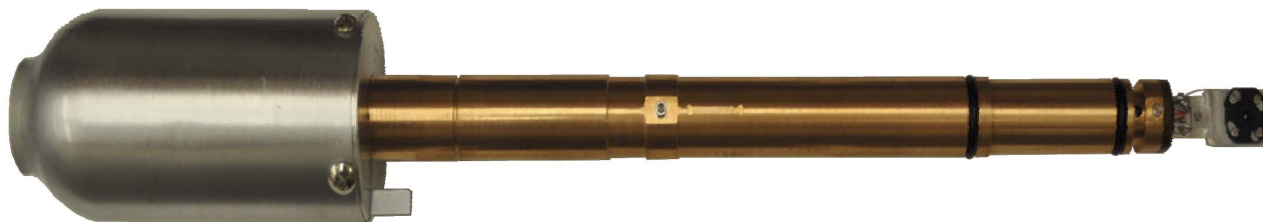
FIG. 1. Image of the environmental wet cell used for this study, which is assembled simply with O-rings and screws, and utilized commercial silicon nitride grids as the substrates.
