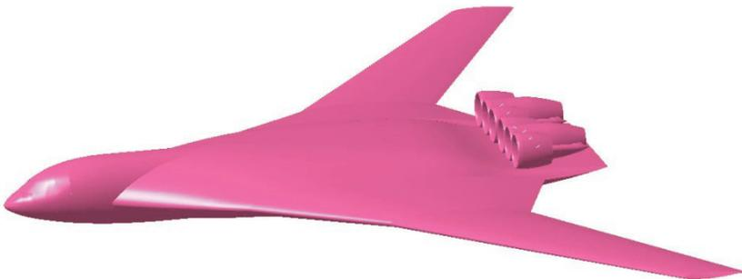
Figure 18. Isometric rendered image of the distributed multiple-fans concept design.
