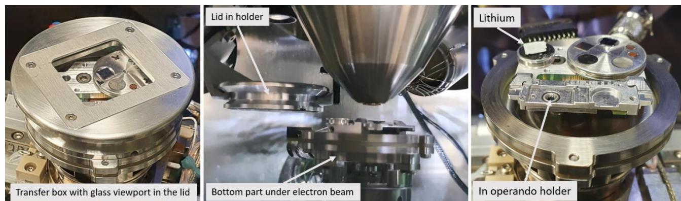
Figure 2. Left: transfer box closed and pumped during transfer from glove box to SEM. Middle: box opened in high vacuum in SEM, sample moved under electron beam. Right: the box contains electrical testing holder and stubs for bulk samples. FIB-SEM battery preparation and in situ testing is possible in the transfer box.
