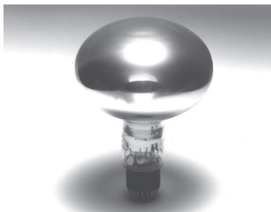
Fig. 5.33. Photograph of an 8-inch photomultiplier (type R 4558) [117].
