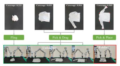
**Figure 1.** FabricFold divides the task of fabric folding into two stages for any given initial configuration. The first stage aims to achieve a relatively smooth fabric by dynamically selecting and executing actions (dynamic or quasi-static) based on the current state of the fabric. The second stage commences once the fabric is sufficiently unfolded and involves performing the folding task by detecting the keypoints of the fabric.
