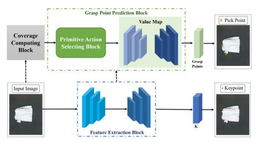
Figure 6. Fabric-folding structure: The RGB image captured by the overhead RealSense 435i camera serves as the input for our system.
