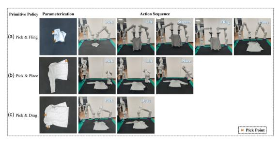
**Figure 4. Primitive actions:** Based on the input received from the overhead RGBD camera, the grasping network can predict a series of pick poses for the upcoming primitive actions.
