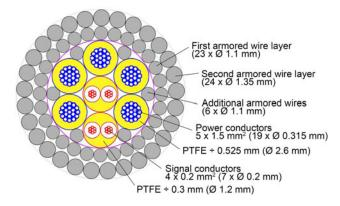
**Fig. 6.** Structure of the armored cable KG  $(5 \times 1.5 + 4 \times 0.2) - 85$ .
