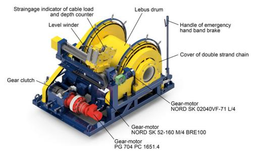
Fig. 4. Structure of the drilling winch.
