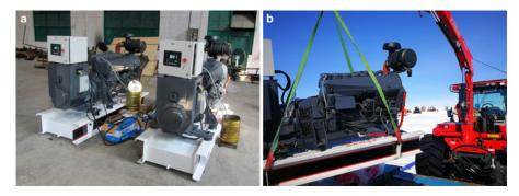
**Fig. 3.** 50-GFNF generators: (a) testing at the factory and (b) unloading into the movable workshop at Zhongshan Station, Antarctica.
