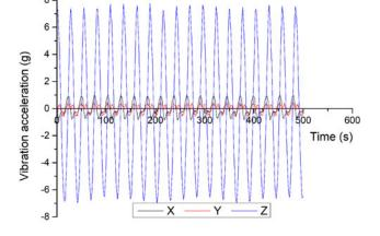
**Fig. 13.** Changes occurring with time in the vibration acceleration in *X*-, *Y*- and *Z*-directions at a frequency of 40 Hz.
