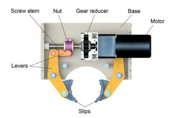
Fig. 8. Structure of the electromechanical clamp.
