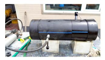
Fig. 16. Pressure testing of casing connections.
