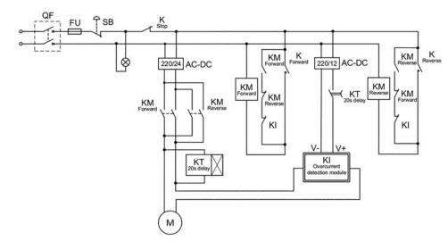
Fig. 9. Electrical schematic diagram of the clamp control system.
