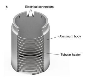
Fig. 17. Thermal casing shoe: (a) structure and (b) heating tests in the lab.
