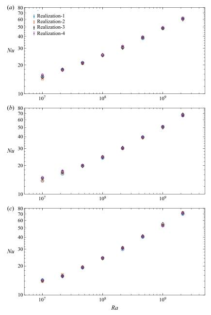
FIGURE 5. Plots of Nu(Ra) data for four different realizations for each p: (a) p = -3.0, (b) p = -2.0 and (c) p = -1.5. The first realizations for the different values of p are generated using the same set of  $\phi_k$  (see (3.2)). The error bar on each Nu data point represents the standard deviation of the averaged Nu calculated from eight different horizontal sections.
