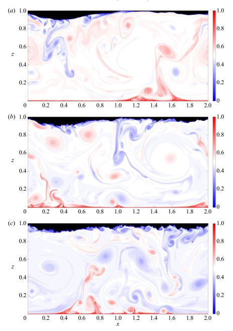
FIGURE 2. Temperature fields at t = 100 for  $Ra = 2.15 \times 10^9$  and (a) p = -3.0, (b) p = -2.0 and (c) p = -1.5. (See also the movies in the supplementary material available at https://doi.org/10.1017/jfm.2020.826.)
