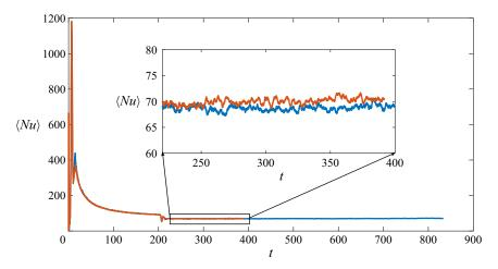
FIGURE 9. A 200 time-unit moving average of the Nu(t) data measured at z/H = 0.42 for two simulations of different duration with the same roughness profile, p = -1.5 and  $Ra = 2.15 \times 10^9$ .
