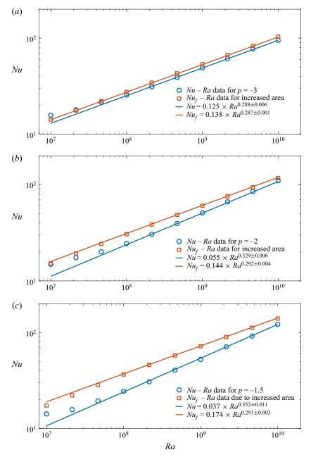
FIGURE 13. Heat flux data for the fractal boundaries (*Nu*) and theory that applies heat flux for flat boundaries over an augmented area (*Nu<sub>f</sub>*): (a) p = -3; (b) p = -2; and (c) p = -1.5. The power-law fits are for the range  $Ra \in [10^8, 10^{10}]$ .
