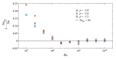
FIGURE 4. Residuals of the power-law fits shown in figure 3 for p = -3.0, -2.0 and -1.5. Here,  $Nu_{fit}$  are the values of the Nusselt number obtained from the power-law fits for the range  $Ra \in [10^8, 10^{10}]$ .
