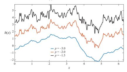
FIGURE 1. Functions used for the upper surface of the convecting domain generated using (3.2) for different values of p and for  $\mathcal{K} = 100$ . The degree of roughness increases as the value of p increases. The curves are vertically displaced by 2 units to improve their visibility.
