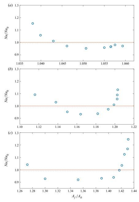
FIGURE 12. Plots of  $Nu/Nu_0$  versus  $A_f/A_0$  for: (a) p = -3; (b) p = -2; and (c) p = -1.5.
