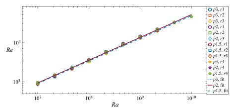
FIGURE 7. Plot of Re(Ra) data for all p and the different realizations denoted r1-r4. The power-law fits shown here are those reported in figure 6 for  $Ra \in [10^7, 10^{10}]$ .
