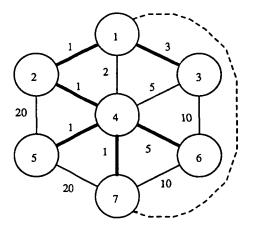
Suppose that the pressure at node number 1 is set at 1, and the pressure at node 7 is set at 0. The relation between the flow q and the pressure difference p is given by
