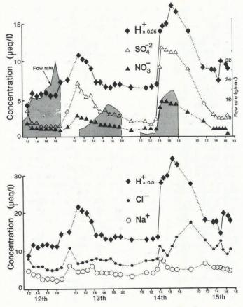
Fig.4. Meltwater concentrations for five major ions at the 1.8 m nest over the 4 days of the melt experiment. Time in hours on each day is shown. H<sup>+</sup> is shown on both graphs for comparative purposes but note the change in the ordinate scale.
