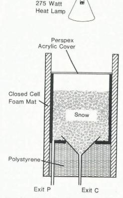
Fig.2. Experimental configuration for the laboratory melt experiments. The inner cylinder has a diameter of 25 cm and a height of 30 cm.
