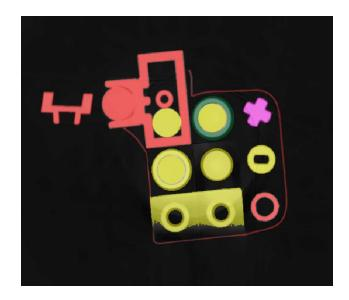
Figure 1. Lego sample segmented into different types of plastic.
