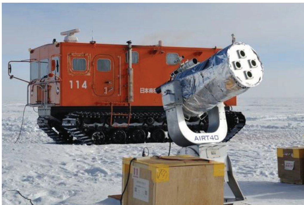
The Tohoku-DIMM placed on the mount for the AIRT 40 cm infrared telescope at the Japanese Dome Fuji Station at Dome F. Credit: Hirofumi Okita
