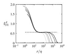
FIGURE 4. Scaling exponent  $\xi_{[4]}^E$  for the cases R1–R6 with  $Re_{\lambda}$  ranging from 119 to 754 (higher Reynolds numbers indicated by darker shading). The dashed black horizontal line indicates  $\xi_{[4]}^E = 0.56$ .
