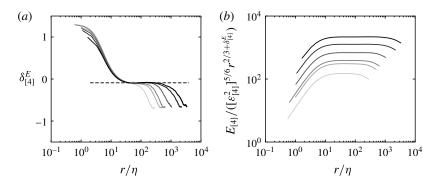
FIGURE 6. The term  $\delta^E_{[4]}$  as evaluated by (4.12) for R1–R6 (a). Plot of the ratio  $\langle E_{[4]} \rangle / (\varepsilon^2_{[4]} r^{2/3 - \delta^E_{[4]}})$  with  $\delta^E_{[4]} = -0.09$  (b). Higher Reynolds numbers are indicated by darker shading.
