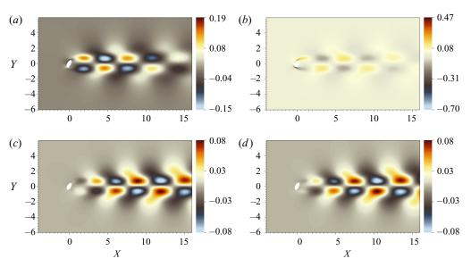
FIGURE 15. Streamwise velocity component of the eigenvector for (a,b) vertical oscillation and (c,d) rotational FSI cases. The left panels show the real part of the eigenvector and the right panels show the imaginary part of the eigenvector corresponding to the unstable eigenvalue.
