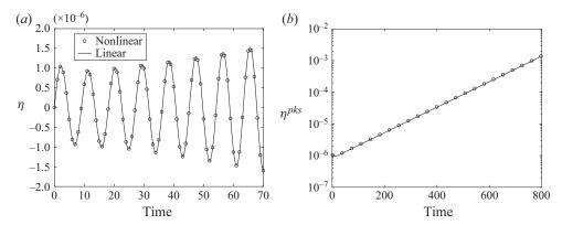
FIGURE 3. Comparison of linear and nonlinear evolution of cylinder position  $\eta$  for identical small-amplitude disturbance. (a) The time evolution of  $\eta$  in the first few cycles of the oscillation. (b) The evolution of peak amplitudes of the oscillation in a semi-log scale.
