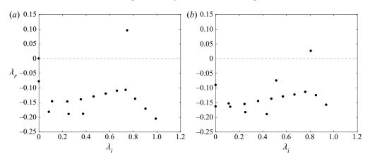
FIGURE 14. One-sided spectra for a rotated ellipse at Re = 50. (a) Spectrum for an ellipse free to oscillate in the vertical direction and (b) spectrum for the ellipse free to rotate about its centre.
