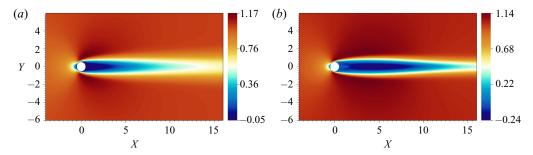
FIGURE 16. Base flow state for a cylinder with splitter plate at (a) Re = 45.0 and (b) Re = 156. Note that the splitter plate is not discernible in the visualization due to its very small thickness (0.02D).
