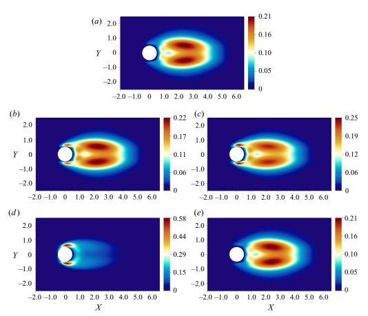
FIGURE 20. Comparison of the structural sensitivity map for the least stable eigenvalue for different values of the natural frequency  $\omega_n$ . The top panel (a) is the structural sensitivity for the stationary cylinder case. The bottom four panels (b-e) represent the cases with FSI. (a) Stationary cylinder; (b)  $\omega_n = 0.0767$ ; (c)  $\omega_n = 0.3833$ ; (d)  $\omega_n = 0.7665$  and (e)  $\omega_n = 3.8327$ .
