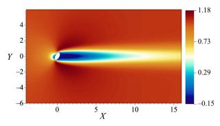
FIGURE 12. Streamwise velocity of the base flow state for a rotated ellipse at Re = 50.
