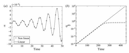
FIGURE 7. Comparison of linear and nonlinear evolution of cylinder position  $\eta$  at Re=40 and  $U^*=8$ . (a) Time evolution of  $\eta$  in the first few cycles of the oscillation. (b) Evolution of peak amplitudes in a semi-log scale.
