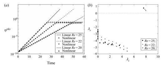
FIGURE 10. (a) Comparison of linear and nonlinear evolution of peak amplitudes vertical displacement  $\eta$  for a confined cylinder at three different Reynolds numbers. (b) One-sided eigenvalue spectra for the three different Reynolds number cases.
