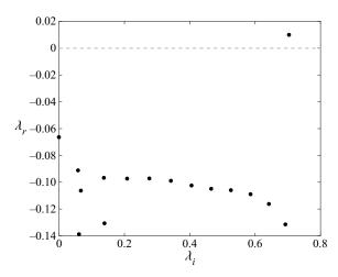
FIGURE 4. One-sided eigenspectrum for a cylinder in cross-flow at Re = 23.512.
