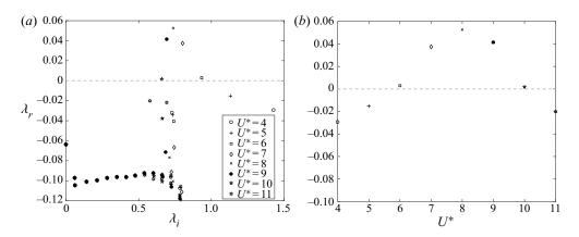
FIGURE 8. (a) One-sided spectra for an oscillating cylinder at Re = 40 for varying reduced velocities  $U^*$ . (b) Variation of the growth rate with reduced velocity  $U^*$ .
